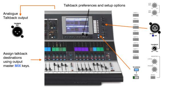
**TB MIC input** Balanced microphone level input. Plug in a wired handheld or gooseneck microphone. If phantom power is required use a pointed object to press in the recessed 48V switch. To avoid thumps make sure the microphone is not live to its destinations when switching phantom power.
